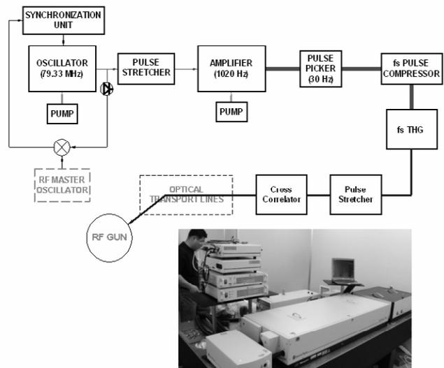
Figure 4: Schematic of GTS laser system.
