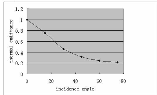
Figure 2: The dependency of the thermal emittance on the (p-polarized) laser incidence angle.
