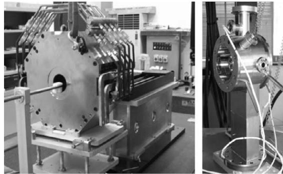
Figure 3: Fabricated GTS solenoid and rf gun.
