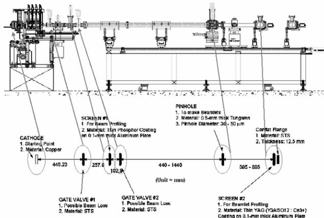
Figure 1: Schematic of emittance meter for measuring the longitudinal profile of beam emittance.
