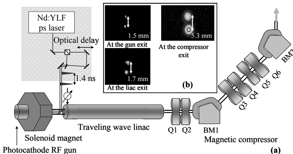
Figure 1: Generation system of double-decker electron beams using a photocathode rf gun.
