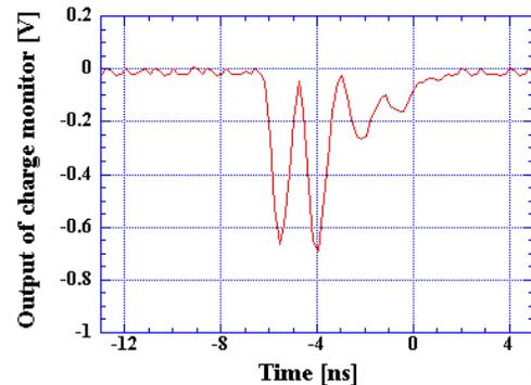
Figure 2: Output of charge monitor downstream of the linac.
