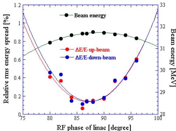
Figure 3: The relative energy spread of the beams as a function of the linac phase.
