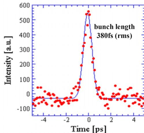
Figure 5: The temporal distribution of the front bunch (up-beam) measured by the streak camera.
