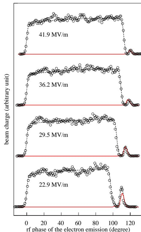
Figure 1: Beam charge vs. the rf phase of the electron emission for different rf input power levels (see text).
