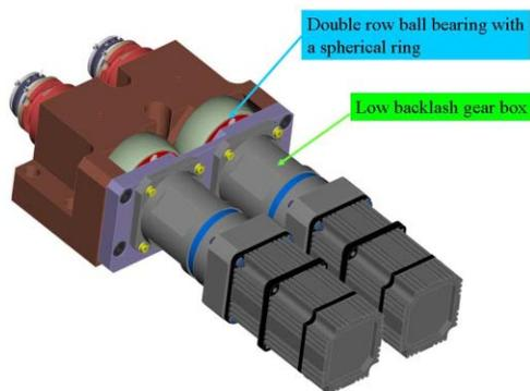
Figure 2: Double cam-shaft mover assembly.
