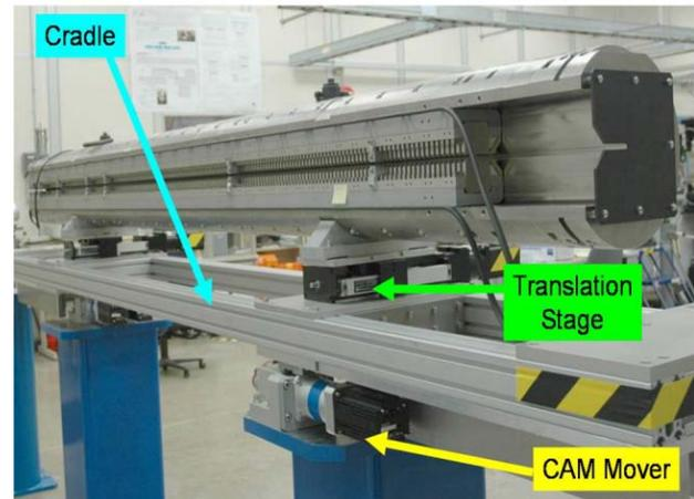
Figure 1: Prototype precision positioning system for the LCLS undulators.
