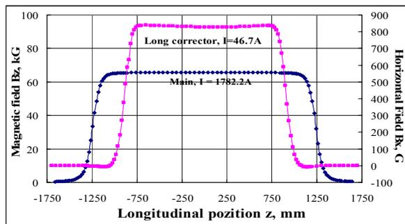
Figure 5: Magnetic field of the main solenoid and the long corrector, each powered on separately.
