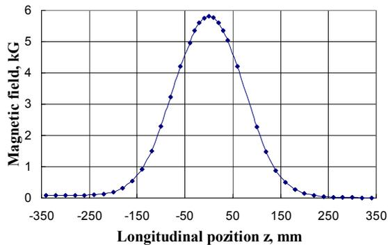
Figure 6: Magnetic field of horizontal short correctors 1.
