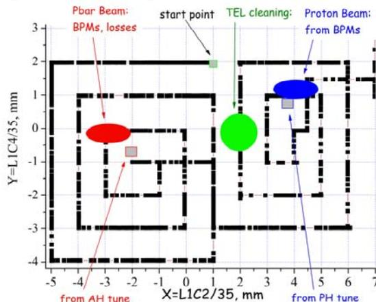
Figure 1: 2-dimensional electron beam position scan around proton and antiproton beams.
