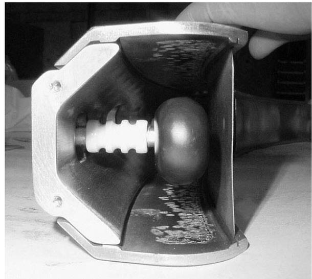
Figure 1: lateral view of the electrostatic deflector.
