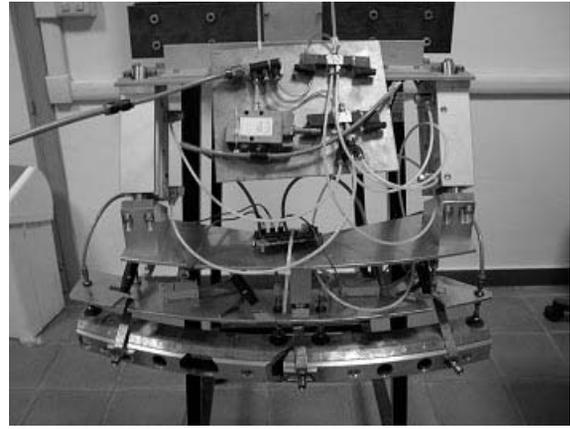
Figure 7: Special device for the remote handling of the CS deflectors.
