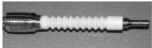
Figure 4: HV Ceramic feedthrough.
