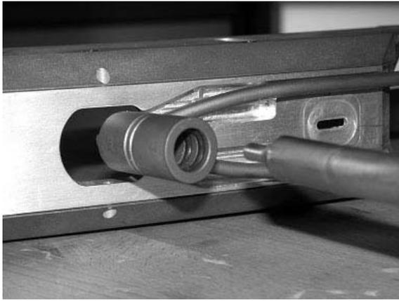
Figure 5: Water feedthrough.
