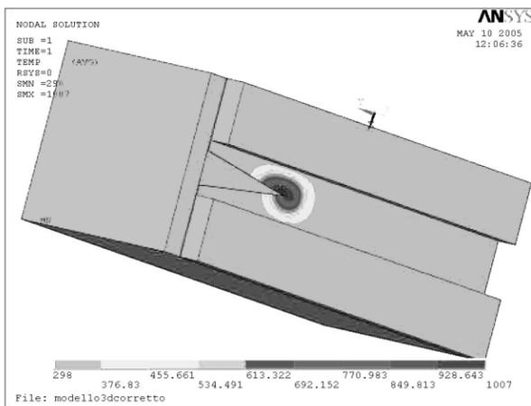
Figure 3: ANSYS simulation of the water-cooled deflector: beam dissipation = 100W.
