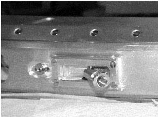
Figure 6: A view of the 'hook' connection.
