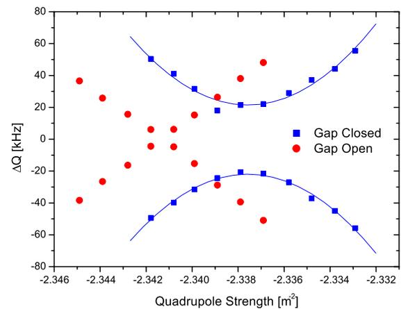
Figure 5: Effect of the wiggler on the beam transverse coupling.
