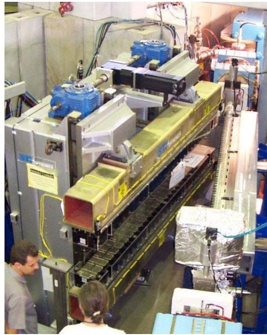
Figure 2: The multipole wiggler being installed in the SR. On the right part of the structure of the vacuum chamber can be seen.
