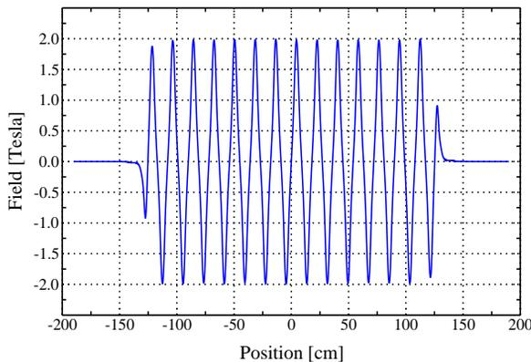
Figure 1: Measured magnetic field along the wiggler magnetic axis.
