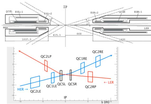
Figure 9: Final quadrupole magnet and compensation solenoids for SuperKEKB (by N. Ohuchi).
