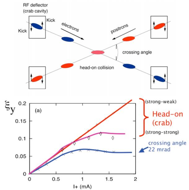
Figure 8: Schematic view of the crab-crossing scheme[6]. On the contrary of the original plan at KEKB, one cavity will be installed in each ring. Though the crabbing orbit propagates over the rings, any problem has not yet been pointed out so far.
