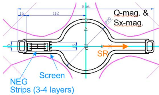
Figure 6: Beam pipe with ante-chamber for SuperKEKB (by Y. Suetsugu et al.).
