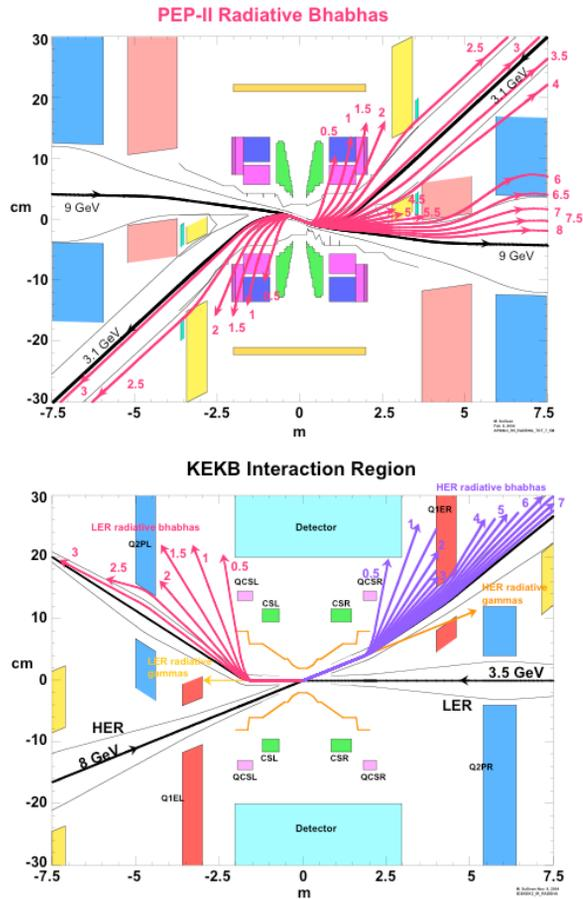
Figure 3: Comparison of the luminosity-dependent detector background due to radiative Bhabha events (by M. Sullivan). Without the crossing angle (upper), this effect is significant.
