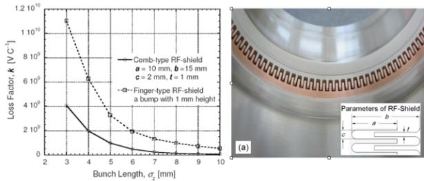
Figure 7: Bellows chamber with comb-type RF shield for SuperKEKB (by Y. Suetsugu et al.). Prototype bellows chambers were installed in the LER at KEKB and showed good performance.
