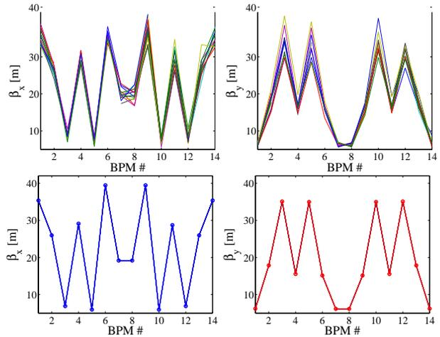
Figure 3: Horizontal (left) and vertical (right) beta functions measured on all BPM of the 16 cells (top) and theoretical values computed from the perfect model (bottom).
