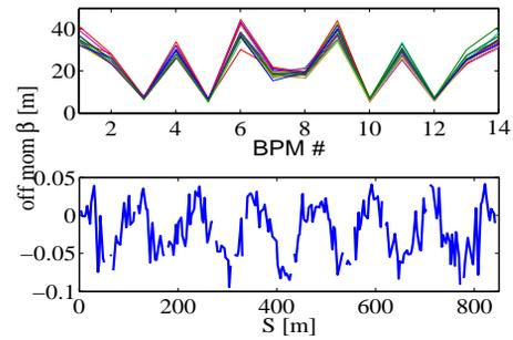
Figure 7: Horizontal off-momentum beta function (top) and corresponding beta variation with respect to on-momentum measurements (bottom).
