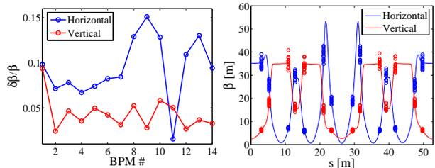
Figure 4: Horizontal (blue) and vertical (red) beta variation measured on all BPM of the 16 symmetric cells (left) and measured beta values (right) from a response matrix analysis (points) as compared to the perfect machine (lines).
