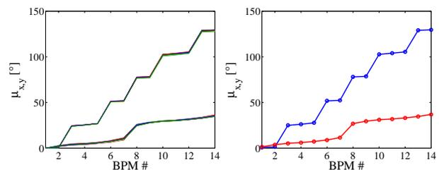
Figure 1: Horizontal and vertical phase advances measured on all BPM of the 16 cells (left) and theoretical horizontal (blue) and vertical (red) values from the perfect machine.
