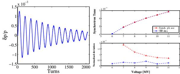
Figure 5: Momentum oscillations issued by a longitudinal kick, recorded on a dispersive BPM (left) and synchrotron tune with respect to the RF voltage (right top) with the associated precision (right bottom), using TBT (blue) and synchrotron phase measurements (red).
