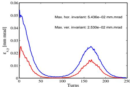
Figure 2: Mean values of the measured horizontal (blue) and vertical (red) transverse invariants for the recorded number of turns.
