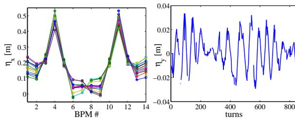
Figure 6: Horizontal (left) and vertical dispersion measured by the TBT data issued by longitudinal kicks.
