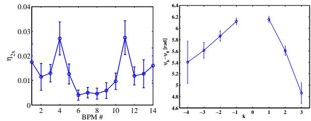
Figure 8: Mean amplitude of the spectral line  $2Q_s$  associated to second order dispersion (left) and phase difference of synchro-betaatron side-bands versus their order (right). The slope is associated to chromaticity.
