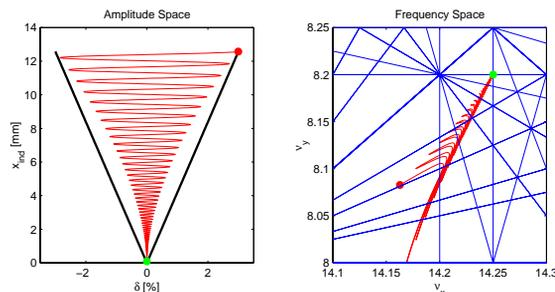
Figure 2: Left: Schematic of particle behavior after Touschek scattering. Initial particle position after being scattered (red dot) then oscillating in energy and amplitude (red line) and damping back to the closed orbit (green dot). Right: particle trajectory in tune space, resonances up to fifth order are shown.
