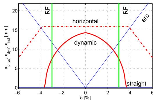
Figure 1: Contributions of the different apertures to the total momentum aperture as a function of the relative momentum deviation  $\delta$ . The thin blue lines represent the induced amplitudes, for an arc or a straight section of the ring. Dashed-dotted red lines stand for the physical apertures, and the vertical green lines show the RF-momentum aperture. This figure as well as the following ones is plotted at the injection point ( $\beta_x(s_0) = 12$  m).
