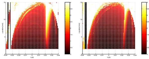
Figure 10: Maximum vertical amplitude reached when tracking particles for 1024 turns. Left: Case with high coupling. Right: Case with low coupling and dispersion wave. The vertical emittance is identical in both cases.
