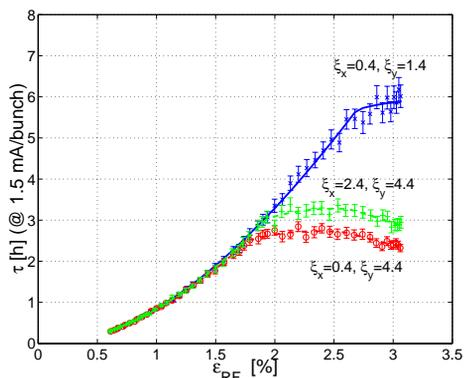
Figure 4: Measurement of the beam lifetime as a function of the RF-momentum aperture for three different sets of chromaticities. One can see that the dynamic momentum aperture has a severe impact on the overall momentum aperture and therefore the Touschek lifetime.
