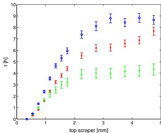
Figure 9: Measured lifetime of the ALS versus half aperture in one straight for three different cases: excited coupling resonance (red), corrected coupling and vertical dispersion (green), vertical dispersion wave (blue). The two cases with excited coupling resonance and dispersion wave were measured for identical vertical emittance.
