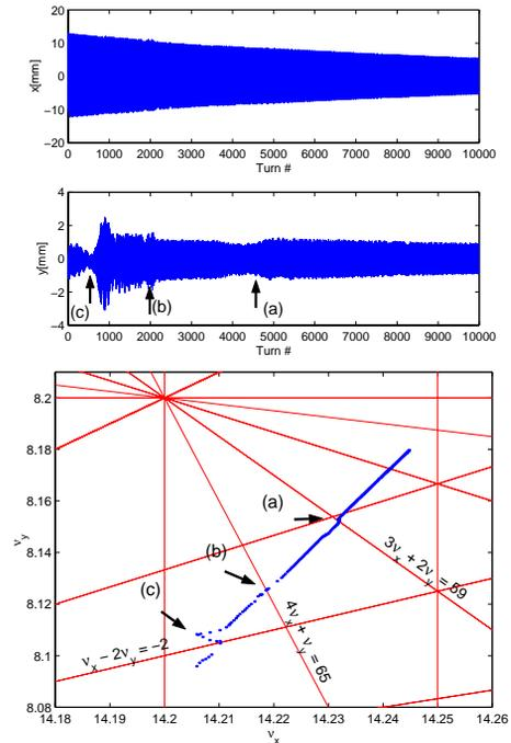
Figure 3: Tracking of particle with synchrotron oscillations and radiation damping. When the trajectory crosses a region with high diffusion (see labels (a) to (c)), the vertical oscillation amplitude increases and at (c) the particle gets very close to the physical aperture of 4 mm.
