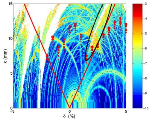
Figure 8: Simulation of a frequency map with the energy offset and the horizontal oscillation amplitudes as the variables spanning the configuration space. The color code indicates the diffusion rate on a logarithmic scale.
