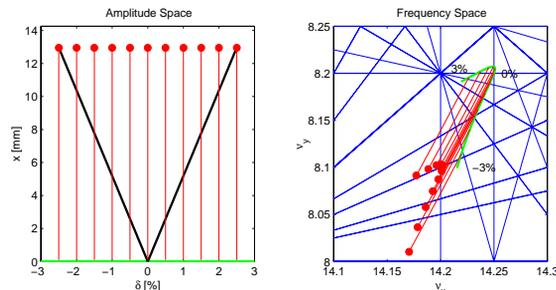
Figure 5: Schematic of the measurement technique to study the off-momentum dynamics. The particle (red dot) damps down to the closed orbit (green line) without synchrotron oscillations. Left: configuration space with induced amplitude after a Touschek scattering (black lines). Right: tune space.
