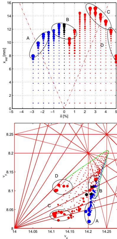
Figure 6: Measurement data showing the relative beam loss in configuration space (upper plot) and in tune space (lower plot) for the low chromaticity case. The dot thickness corresponds to the amount of normalized beam loss. The solid green line marks the tune shift with energy for particles with very small oscillation amplitudes.
