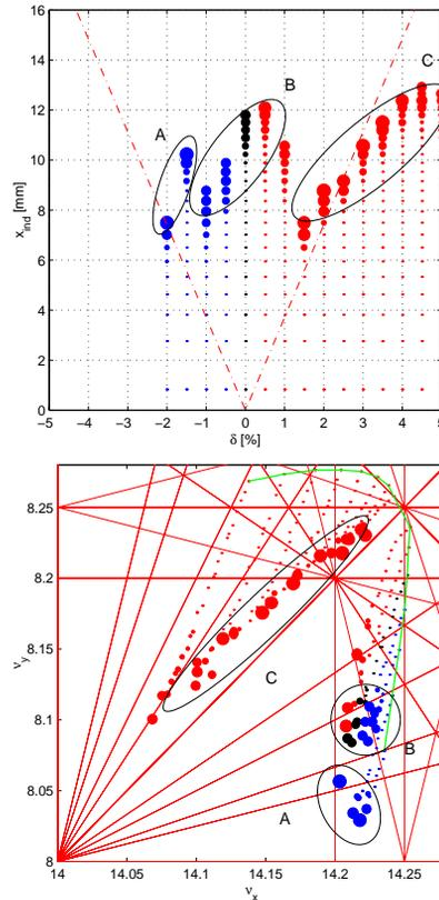
Figure 7: Measurement data for the case with higher vertical chromaticity. Significantly different areas of the tune space are sampled compared to the low chromaticity case.
