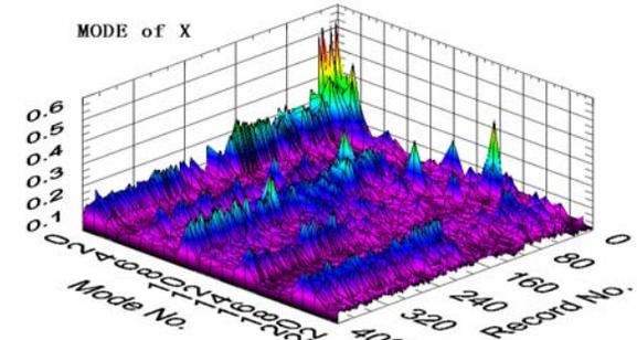
Figure 7: Mode display in X-direction.
