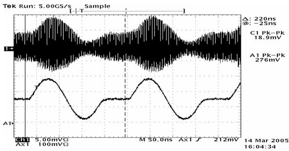
Figure 4: Modulation signal and simulation beam signal.
