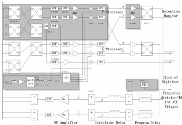
Figure 1: An overview of the transverse feedback system.
