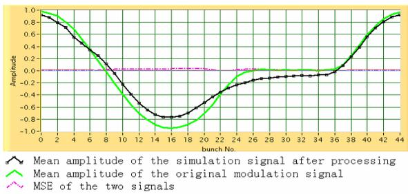
Figure 5: Simulation beam signal detected by ADC.
