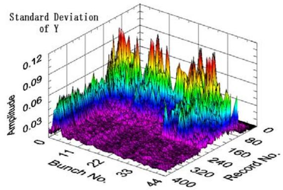
Figure 10: Standard Deviation of beam position in the Y-direction.
