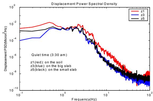
Figure 5: PSDs of vertical vibrations on ground and slabs.
