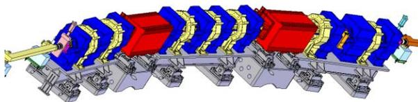
Figure 3: A storage ring cell assembly.
