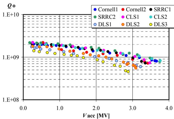
Figure 2: Vertical test results of ACCEL produced cavities.
