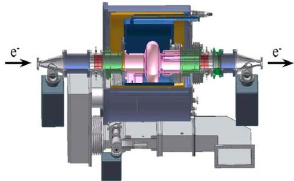
Figure 1: CESR-type cryomodule for TLS.
