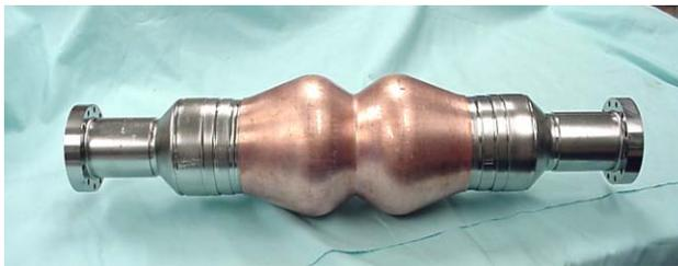
Figure 6: Picture of the completed Nb/Cu cavity.
