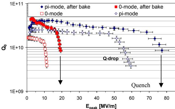
Figure 2:  $Q_0$  vs.  $E_p$  for the two-cell cavity measured at 2 K before and after baking at 120 °C for 48 h.
