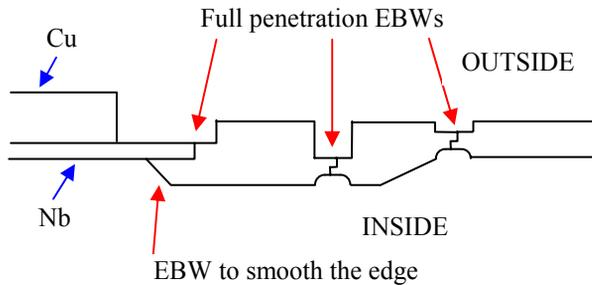
Figure 5: Schematic of adaptive rings used to join the cavity to the niobium beam pipes.
