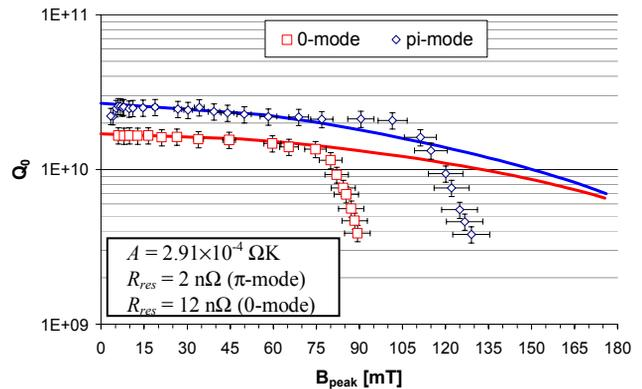
Figure 3:  $Q_0$  vs.  $B_p$  data before baking compared with the thermal feedback model (solid lines).
