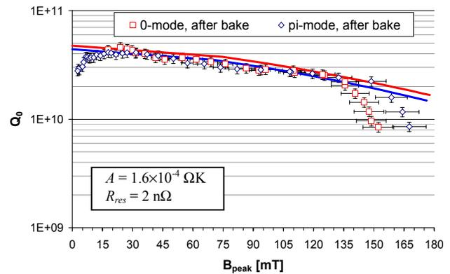
Figure 4:  $Q_0$  vs.  $B_p$  data after baking compared with the thermal feedback model (solid lines).
