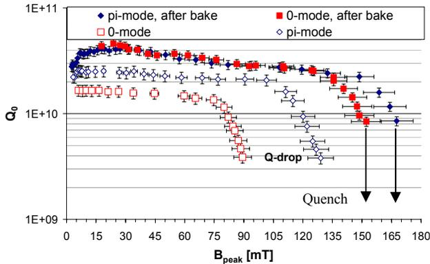
Figure 1:  $Q_0$  vs.  $B_p$  for the two-cell cavity measured at 2 K before and after baking at 120 °C for 48 h.
