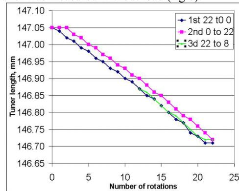
Figure 6: Blade tuner elongation measurement
