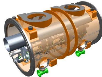
Figure 1: Cryomodule design for 4 cavities.
