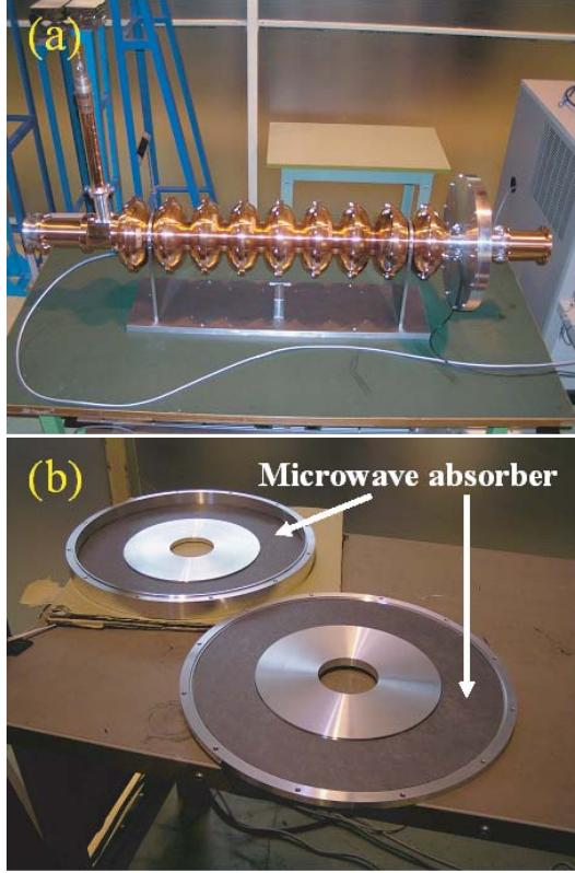
Figure 2: (a) A low-power model of 9-cell TESLA-type cavity with a radial-line HOM damper. (b) Inside of the radial-line HOM damper.
