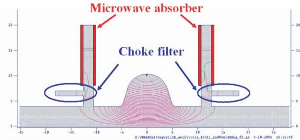
Figure 1: Conceptual design of the radial-line HOM damper.
