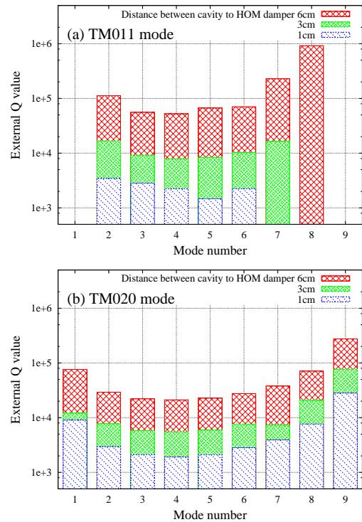
Figure 4: Measured  $Q_{\text{ext}}$  for the (a) TM011 and (b) TM020 modes. The red, green and blue bars indicate the results under the conditions of (2), (3), and (4), respectively.
