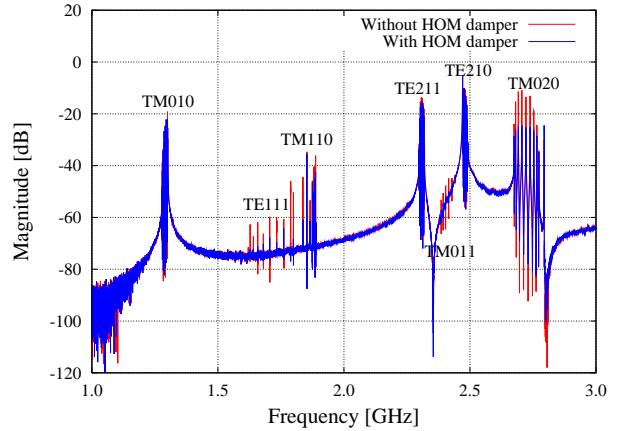
Figure 3: Mode spectra of the 9-cell model cavity. The blue and the red lines indicate the cases with and without the HOM damper, respectively.
