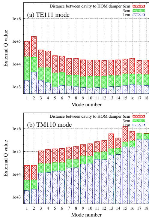
Figure 5: Measured  $Q_{\text{ext}}$  for the (a) TE111 and (b) TM110 modes. The red, green and blue bars indicate the results under the conditions of (2), (3), and (4), respectively.
