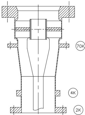
Figure 5: Cold window subassembly for AMAC TESLA coupler
