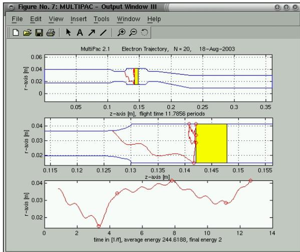
Figure 2: Multipacting trajectories near warm ceramic window at power level 900kW – 1300kW
