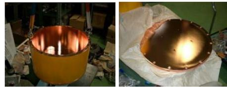
Figure 4: Copper electroplating on the test cavity after EP.
