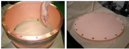
Figure 1: Copper electroplating on the test cavity before EP.
