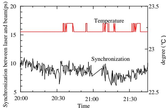
Figure 3: Time evolution of the synchronization and the relevant temperature. The fluctuation of the temperature decreased within 0.1 degrees, and quick and large components in the drift disappears. The jitter in one and a half hours is 600 fs(rms), which is closed to the short time jitter of 340 fs(rms) than previous results (in Fig. 2).
