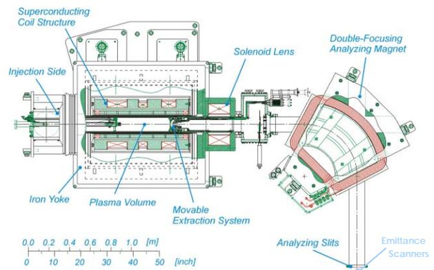
Figure 1: Mechanical layout of VENUS and its accompanying transport system.
