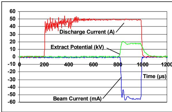
Figure 6: Scope traces for 10A Penning coil current.
