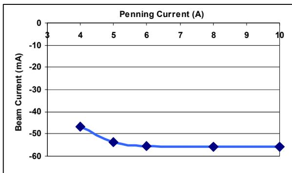
Figure 7: Variation of output beam current with Penning current.
