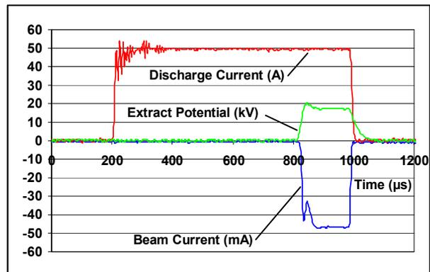
Figure 5: Scope traces for 4A Penning coil current.
