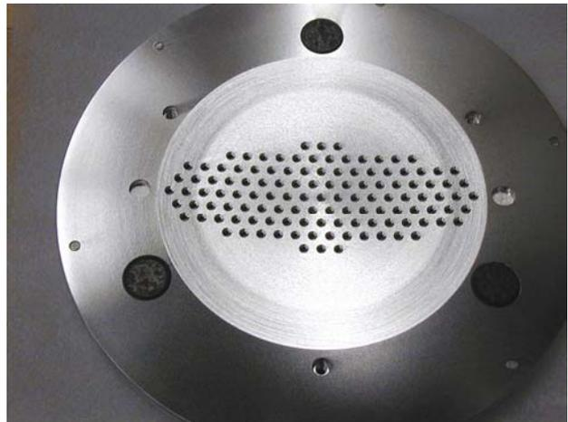
Figure 3: One of the Lens Plates with 119 beamlet holes. The radius of curvature is about 60 cm.
