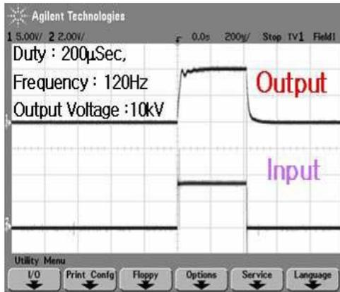
Fig. 4: Output voltage of the fast high voltage switch.
