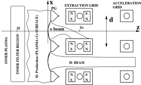
Figure 1: Typical extraction geometry (not to scale): PG = plasma grid; circles are cooling water channels
