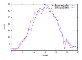
Figure 1: Horizontal IPM beam profile compared with Synergia simulation results passed through our IPM simulation.
