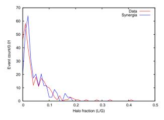
Figure 3: Distribution of L/G values near injection in a single Booster cycle, compared with the distribution of L/G values from a Synergia simulation.
