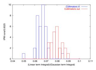
Figure 4: Distribution of L/G values in the Booster with and without collimators.
