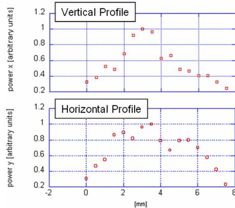
Figure 2: Beam profile measurements of the THz beam
