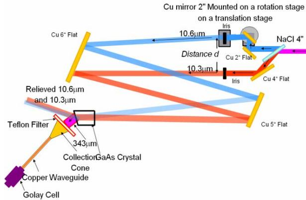
Figure 4: Schematic of High Power Optical Setup
