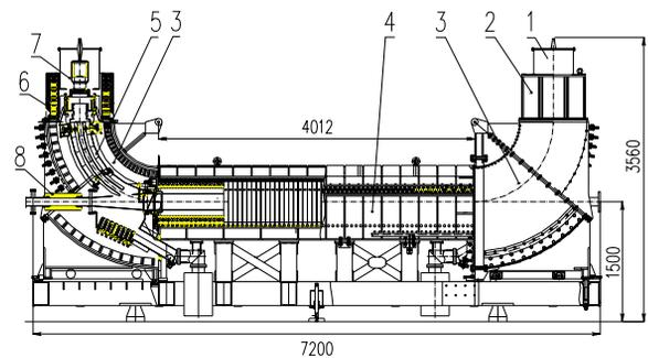
1. E-gun, 2. Solenoid of gun, 3. Toroid, 4. Main solenoid,
