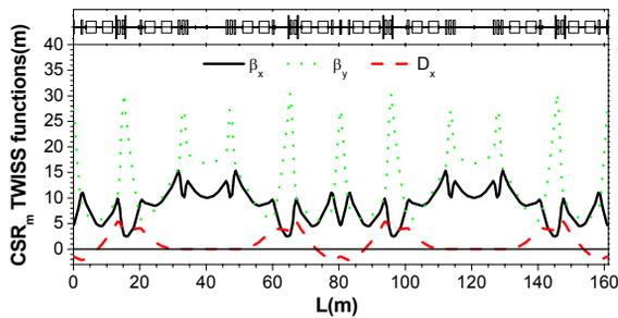
Figure 4:  $\beta$  and dispersion of CSRm
