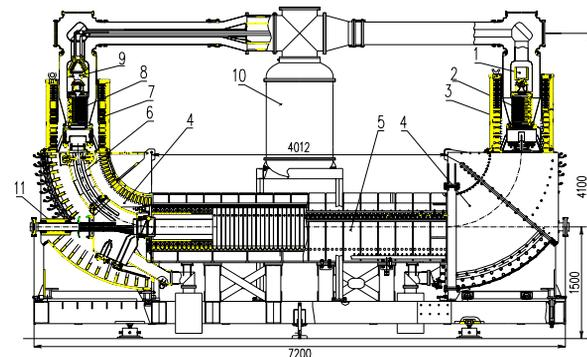
1. E-gun, 2. Accelerating tube, 3. Solenoid of gun,
