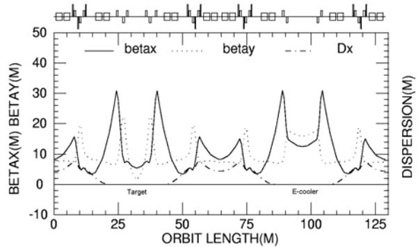
Figure 6: Twiss functions of CSRe.
