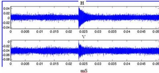
Figure 17: Injection kicker transient recorded with turn-turn BPMs. The BPMs are also used to study non-linear beam dynamics.
