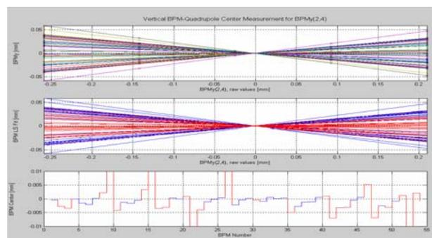
Figure 7: BPM electrical centers are measured with a quadrupole modulation system having a resolution of order 10μm. Beam is moved horizontally and vertically in a quad adjacent to the BPM while the quad strength is varied by ~1% until BPMs elsewhere in the ring show no orbit variation as indicated by “bow-tie” plots (top two graphs). The resulting BPM readings give offsets (lower) that are subtracted from orbit measurements.
