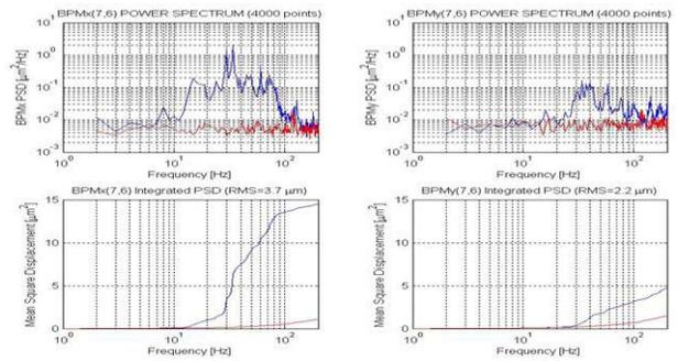
Figure 6: Horizontal (left) and vertical orbit noise spectra, with beam (blue) and without (red), up to 200 Hz detected with electron BPMs. Integrated noise as shown is ~2% of the horizontal beam size and ~10% of the vertical beam size. Peaks <100 Hz are associated with known magnet vibration modes.
