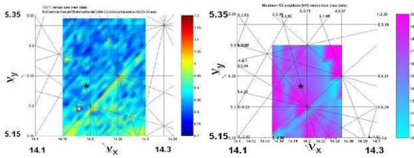
Figure 12: The working point ( $v_x=14.19$ ,  $v_y=5.23$ ) was optimized by measuring dynamic aperture (left, by increasing horizontal kicker amplitude until beam lost) and lifetime (right) as a function of tunes. The main resonance line is  $v_x - v_y = 9$ .
