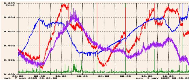
Figure 8: Vertical rms orbit over 48 h is held to <1 μm by feedback (green) while beam line photon monitors (red for bend magnet line, blue for undulator line) indicate diurnal orbit motion correlated with the temperature of BPM processors (violet, 6°C pk-pk). Glitches in rms orbit are caused by traffic on the trestle over the ring and during injection.
