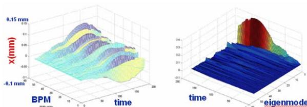
Figure 5: Horizontal orbit drift over 10 hours (left) is on the order of 100 μm. Orbit distortion is decomposed analyzed into eigenmodes of the response matrix (right) and used for orbit feedback.
