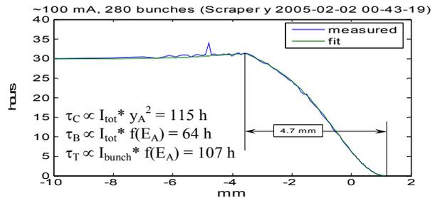
Figure 16: Coulomb, bremsstrahlung and Touschek lifetimes ( $\tau_C$ ,  $\tau_B$ ,  $\tau_T$ ) are derived from total lifetime measurements at as a function of vertical scraper position for two fill patterns: 100 mA in 280 bunches and 20 bunches. Knee in curve indicates vertical aperture  $y_A$  is 4.7 mm elsewhere in ring.  $E_A$  designates energy aperture.
