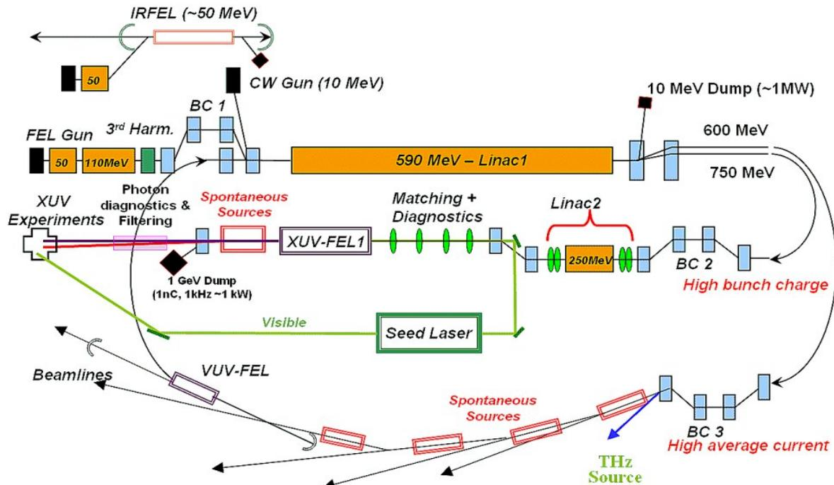
Figure 2: Possible baseline layout scheme for 4GLS
