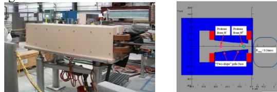
Figure 7: Photograph and model of the injection dump gradient magnet.
