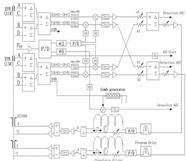
Figure 1: Overview of the BxB system of the HLS.
