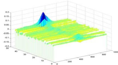
Figure 9: BxB Recording of single bunch exciting.
