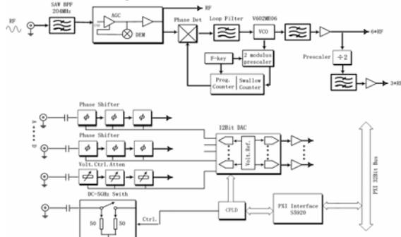
Figure 2: PLL freq-multiplier and RF controller.
