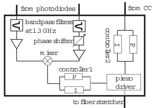
Figure 2: Schematic of the electronic feedback circuit.
