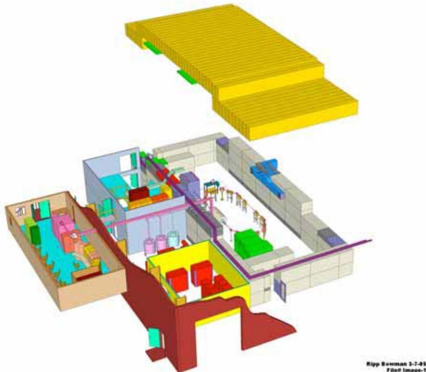
Fig.1 The layout of the R&D ERL facility in the bay of Bldg. 912 at BNL. The bay is equipped with an overhead crane. The facility has a control room, two service rooms and a shielded ERL cave. The control room is located outside of the bay in a separate building. The single story house is used for a high voltage power supply for 1 MW klystron. The two-story unit houses a laser room, the CW 1 MW klystron with its accessories, most of the power supplies and electronics
