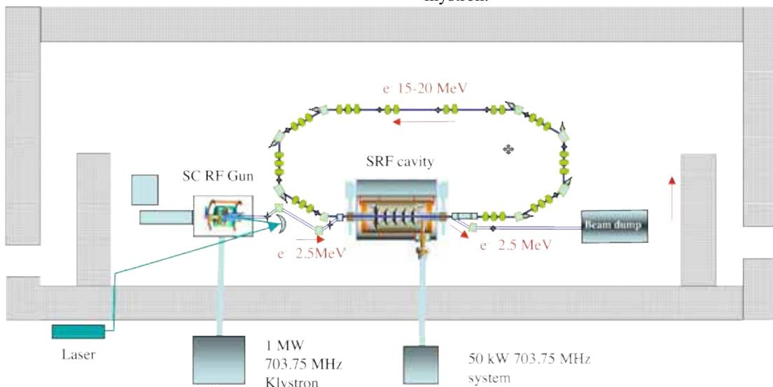
Fig. 2 Layout of the R&D linac in the shielded vault
