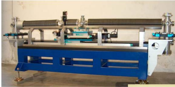
Figure 5: Emittance-meter device with long bellows.
