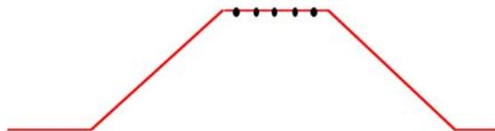
Figure 1: Schematic view of an extraction pulse with an extended flattop suitable for extracting 5 evenly spaced bunches. Rise and fall times are roughly equal and the flattop is a bit more than half the rise time.
