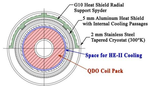
Figure 4: QD0 Cryostat Detail at Support Location.
