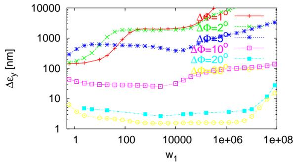
Figure 3: The emittance growth for different phase shifts.
