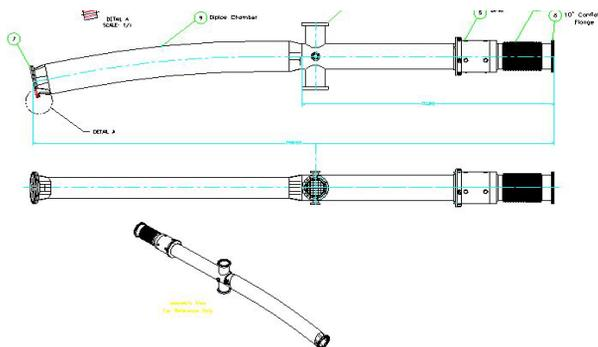
Figure 3: Typical half-cell vacuum chamber assembly.
