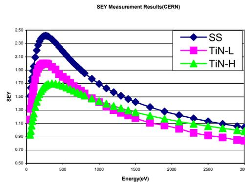
Figure 6: SEY as a function of incidence electron energy for bare and TiN coated stainless steel coated at high and low pressure.
