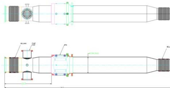
Figure 5: Extraction quad doublet chamber assembly.
