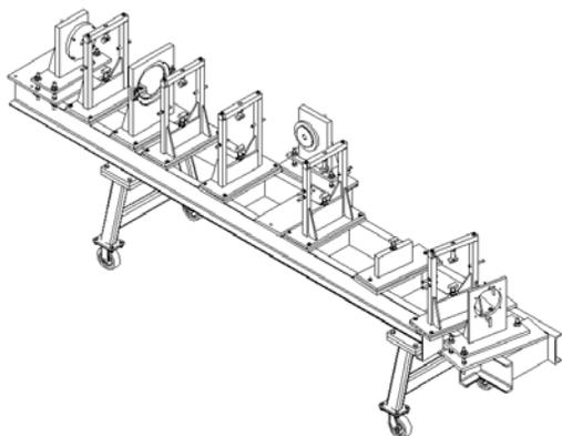
Figure 2: Fixture used to align chambers during welding.
