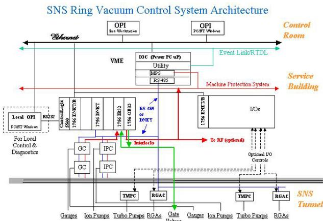
Figure 7: I&C Vacuum system schematic.
