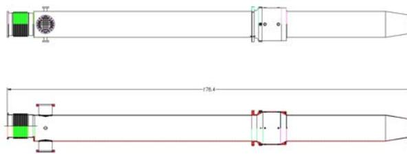
Figure 4: Injection quad doublet chamber assembly.
