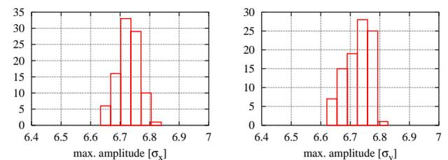
Figure 1: Results of a Monte-Carlo for the protection level of the TCDI system. The LHC is protected at  $6.9 \sigma$ .
