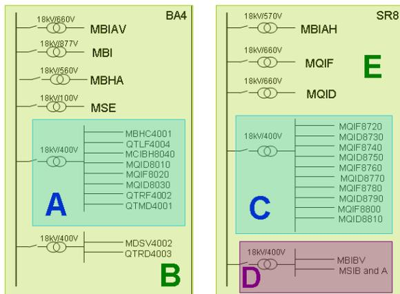
Figure 2: Powering scheme for the magnet families of the injection process via TI 8.
