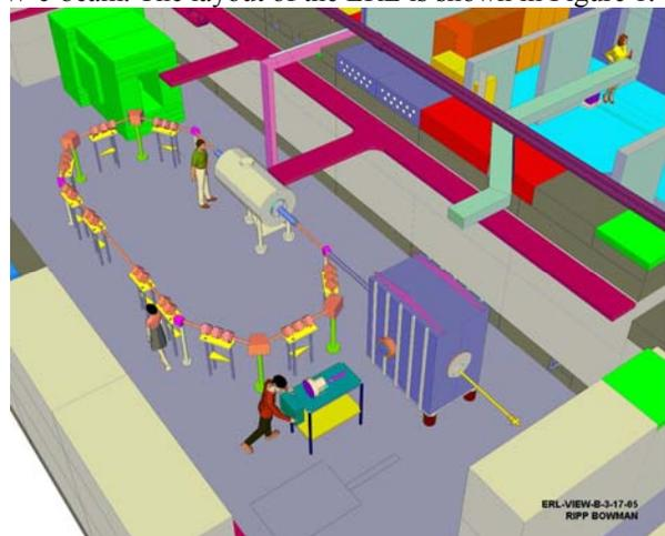
Figure 1: Layout of ERL. The gun is the square structure (blue) on the right, followed by the round 5-cell cavity cryomodule and the beam dump shielding.
