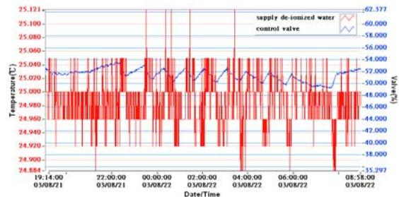
Figure 6: 12-bits control valve vs. temperature variation.
