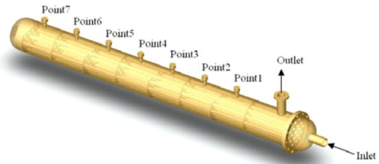
Figure 9: The buffer tank with the compressed volume
