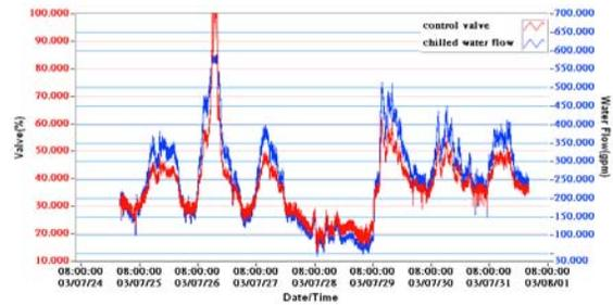
Figure 4: The nonlinear valve vs. water flow variation.
