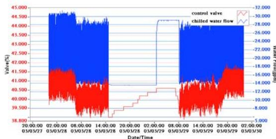
Figure 3: The valve with a backlash gearmotor vs. water flow variation.
