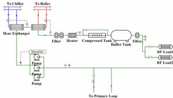
Figure 1: The 2<sup>nd</sup> loop of RF de-ionized water system.
