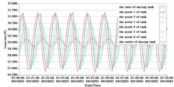
Figure 10: The temperature variation in the compressed buffer tank.
