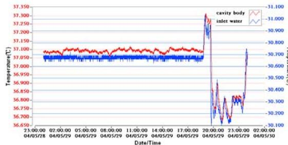
Figure 2: The temperature correlation of the cavity body vs. inlet water.
