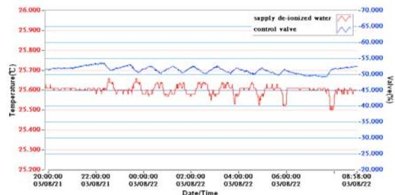
Figure 7: 16-bits control valve vs. temperature variation.
