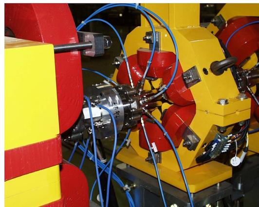
Figure 2: Photograph of the beam energy-spread monitor with eight electrodes.
