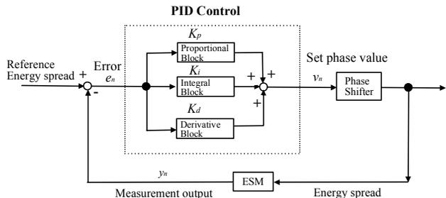
Figure 5: Block diagram of the energy-spread feedback loop.
