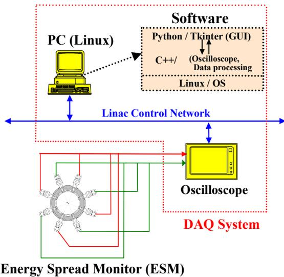
Figure 3: Schematic drawing of the beam energy-spread monitor system.
