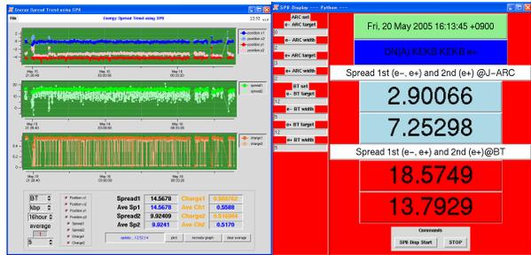
Figure 4: GUI of the energy-spread trend plot (left) and the alarm panel (right).
