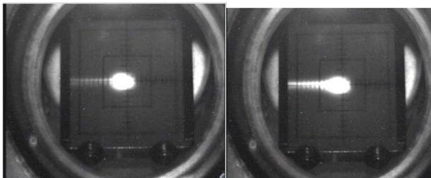
Figure 1: Energy spread measurement using the fluorescent screen monitor in the case of a small energy-spread (left) and a large energy-spread (right) condition.
