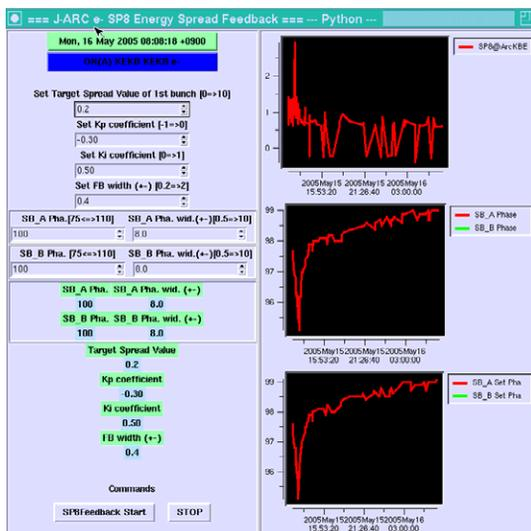
Figure 6: GUI of the energy-spread feedback software.
