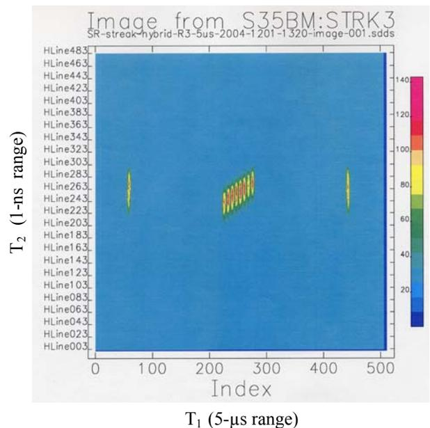
Figure 3: Dual-sweep streak camera image of the hybrid fill using the same ranges as Fig. 2. In this case the singlet is clearly isolated from the eight septuplets. The display does not show the individual members of the septuplets. The singlet has a bunch length of about 50 ps.
