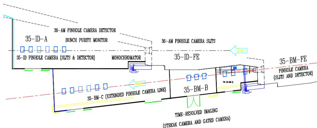
Figure 1: Schematic of the beamlines in Sector 35 dedicated to electron beam diagnostics. The S35 bending magnet (BM) dipole source is used for the OSR detected by the streak camera.
