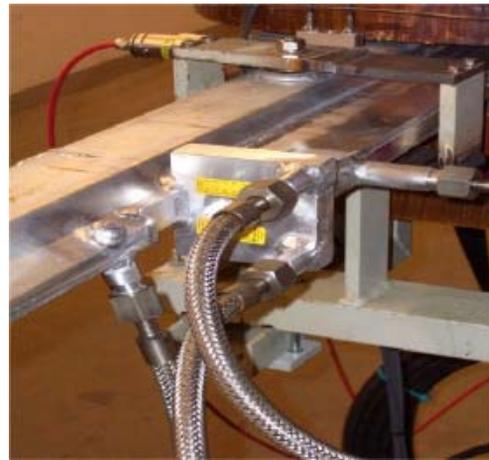
Figure 1: New exit window for Compton photons
