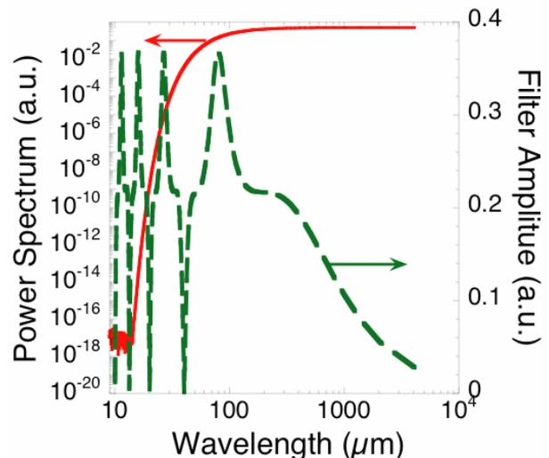
Figure 2: Power spectrum for the CTR of a Gaussian bunch with  $\sigma_z = 20 \mu\text{m}$  (red continuous line) and total transmission spectrum (dashed green line) for the three Mylar foils (see text).
