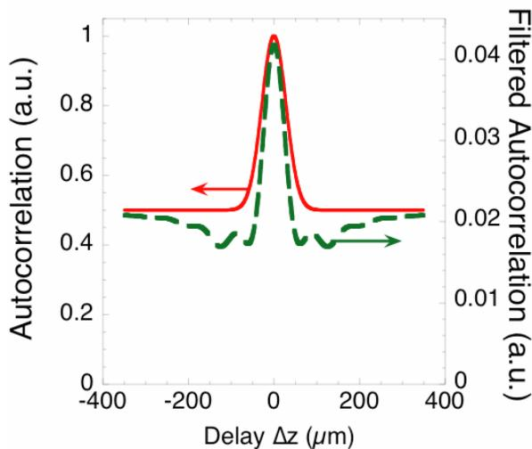
Figure 3: Autocorrelation traces ( $C(\tau)$  in the text) calculated without (continuous red line) and with (dashed green line) the effect of the Mylar foils.
