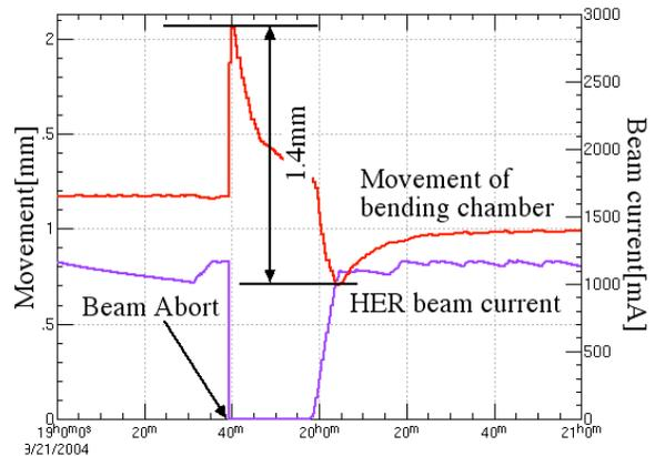
Figure 6: Gap detector measured displacement of bending chamber before and after beam abort in HER
