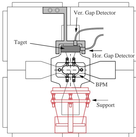
Figure 2: Gap detectors attached to QM
