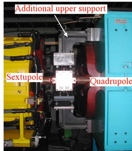
Figure 7: Additional upper support was fixed on a QM
