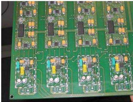
Figure 4: Picture of the four analog channels of the MPRX IV board. DC power supplies and the Bias voltage power supply are not shown.
