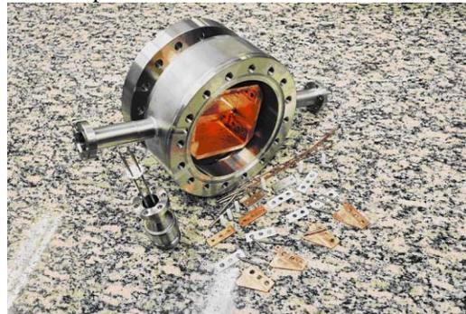
Figure 2: LNLs XR BPM. It is possible to see the electrical feed-through, the blades and the isolating plates and tubes. The mask is mounted in a CF100 flange, the internal aperture for the beam is about 20 mm x 74 mm and the blades are about 25 mm decentralized. As shown in figures 1 and 2, the electrical connector can be installed in two positions, in order to facilitate the installation in different front ends.
