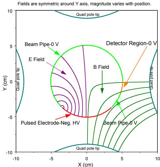
Figure 3: Electric (E) and Magnetic (B) field lines. Note that the picture is rotated 45° to make more efficient use of the display space.
