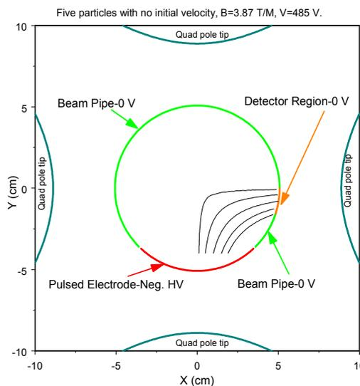
Figure 4: Some swept electron trajectories for electrons of zero initial velocity starting at y = -4 and various x values.
