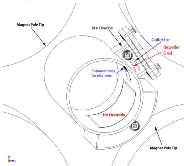
Figure 2: 3D sketch of electron sweeping diagnostic in a PSR quadrupoles.
