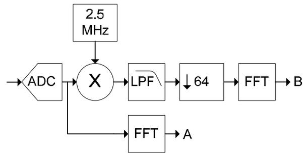
Figure 6: Signal processing chain.
