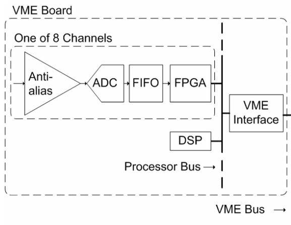
Figure 2: Board level architecture.
