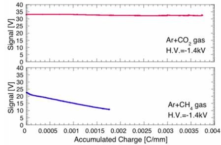
Figure 2: Gain variation due to Co-60  $\gamma$  ray irradiation.
